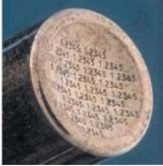
Figure 2. Bullet Using the ACS Marking System [4]
